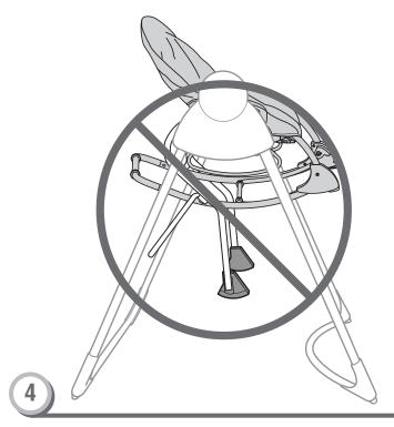
**IMPORTANT!** Do not place the seat on top of the seat tube support! The seat is not secure. Please remove the seat. Re-read and repeat steps 1 - 3.
